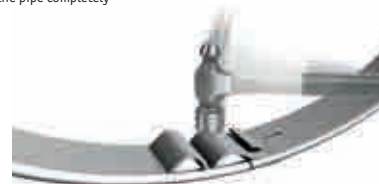
Figure 4 By giving a few taps with a hammer on top of the clamping system the bevel protector expands and forces itself against the inner pipe surface
