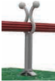
Bottom Hole: Snap-lock \varnothing 4 \pm 0.08 Panel Thickness: 0.8-2
